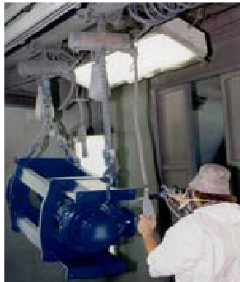
Fig. 5: Explosion-proof mechanical hoist
