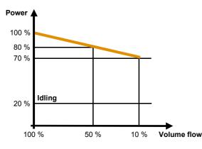
Fig. 6: Control of the volume flow rate using a suction throttle
