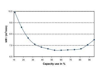
Fig. 5: Specific performance of a speed-controlled compressor
