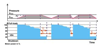
Fig. 4: Range of application peak load compressor
