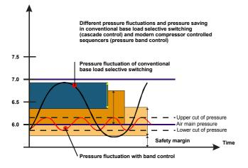
Fig. 9: Pressure band regulation
