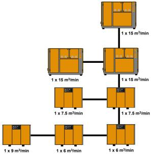
Fig. 10: Ways to split-up compressed air production
