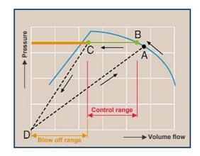
Fig. 7: Turbine bypass control system
