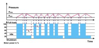
Fig. 2: Range of application peak load compressor
