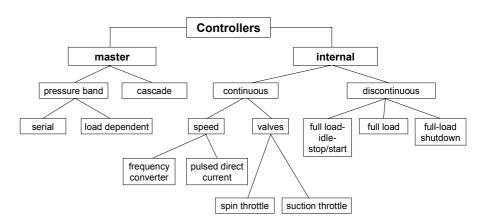
Fig. 1: Control of compressed air systems
