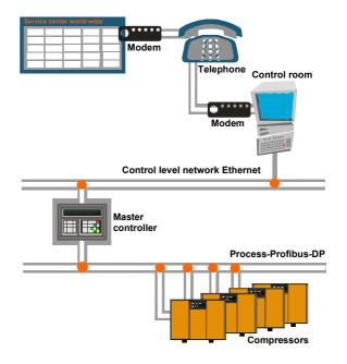
Fig. 11: Use of control technology for compressor control
