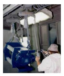
Fig. 5: Explosion-proof mechanical hoist
